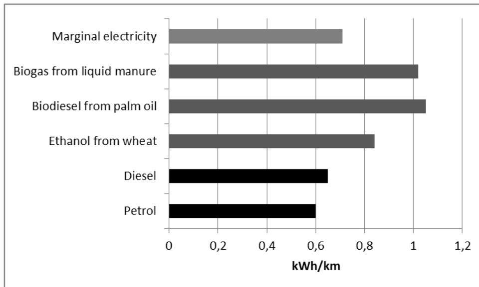
Figure 3 – Primary energy use of BEVs and ICEVs.
