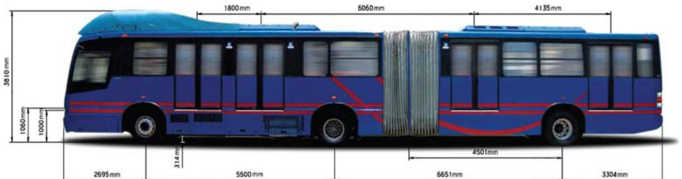
Figure 2 – Vehicle model Volvo BRT 7300
