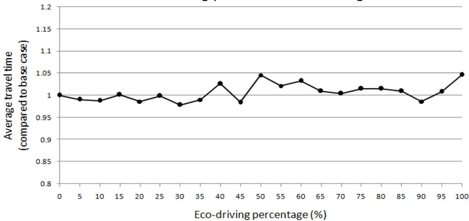
Figure 7 travel time performances with different penetration rates
