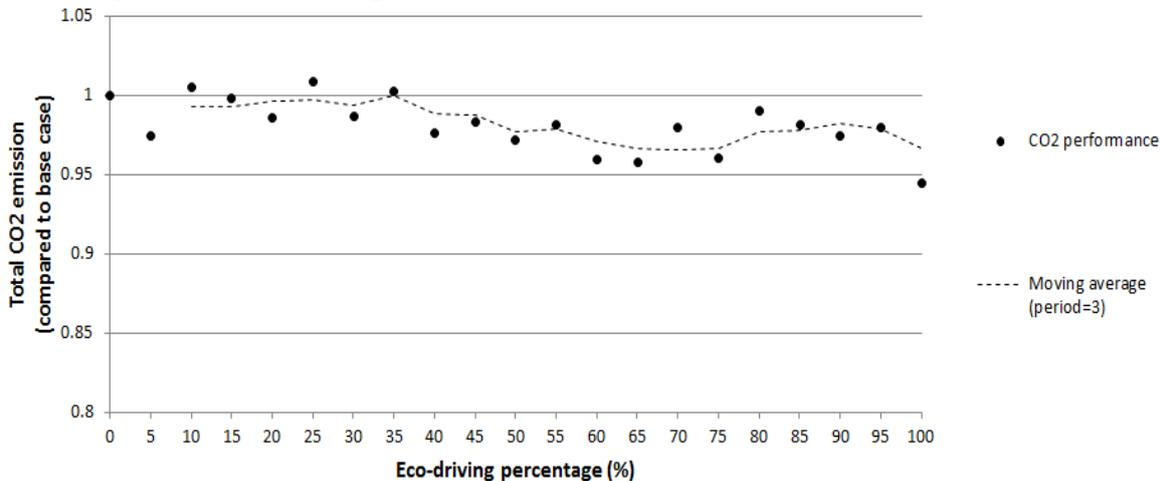
Figure 9 CO2 emission performances with different penetration rates
