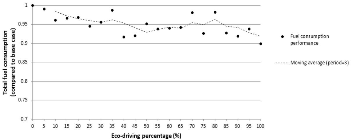
Figure 8 fuel consumption performances with different penetration rates
