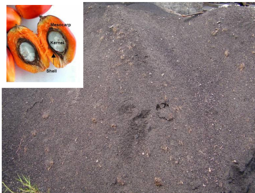
Figure 2.1 - Oil Palm Fruit Ash after burning (inside is fruitlet of palm oil fruit)
