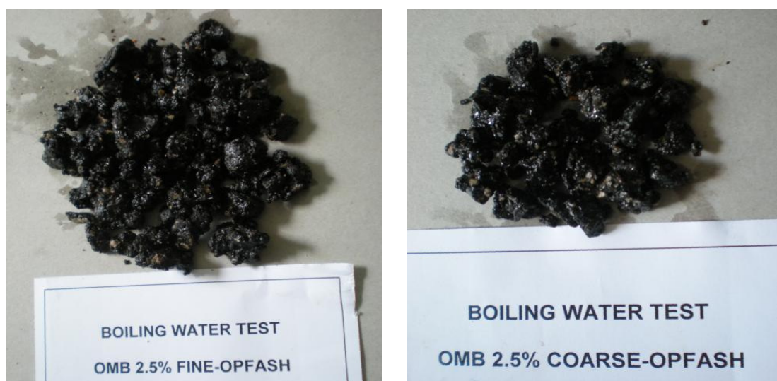
Figure 3.6. - Observe boiling water test for 2.5% F-OPFA-MB (left) and for 2.5% C-OPFA-MB (right)
