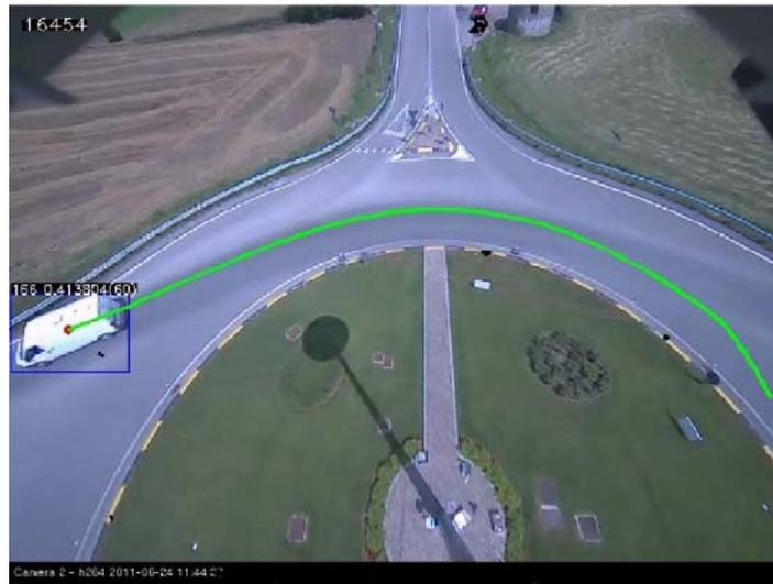
Figure 4: 2D vehicle trajectory extracted on the image plane using the algorithm in (Mussone et al., 2011).
