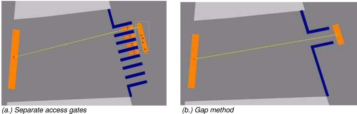
Figure 1 – Turnstile modelling techniques (Source: Hermant *et al.* 2009)
