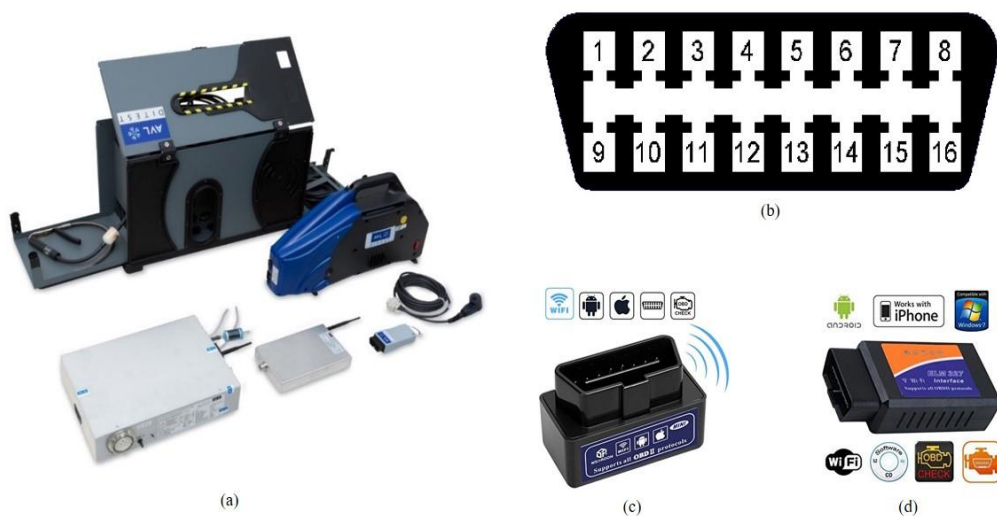
Figure 2. (a) AVL Ditest 1000 instrument (b) OBD data port (c) Bluetooth device and (d) USB device
