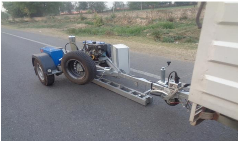
Figure 1. Representation of FWD for evaluation of pavement
