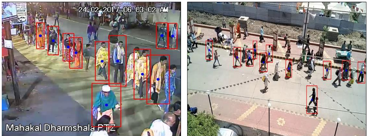
Fig. 4. (a) Pedestrians detected using IPM at Mahakal Dharmshala; (b) Pedestrians detected using IPM in Gao Ghat, Kumbh Mela, Ujjain
