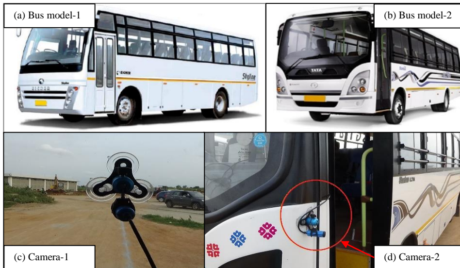
Fig. 1. (a) & (b) Study vehicles used for data collection; (c) & (d) camera positions to record video data.
