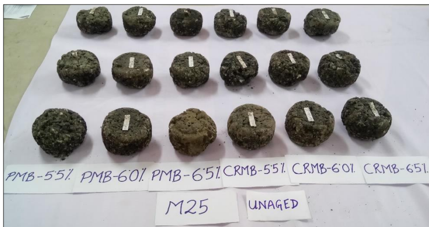
(b) Unaged OGA_25 samples after Cantabro abrasion loss test
