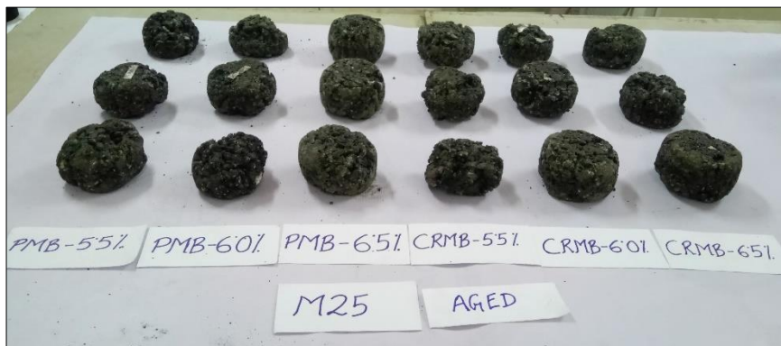
(c) Aged OGA_25 samples after Cantabro abrasion loss test
