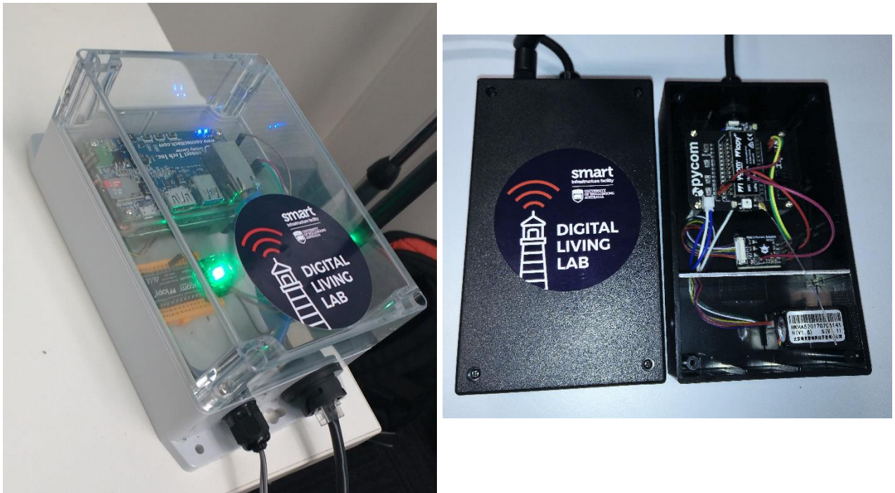
Figure 4 – On the left, the prototype of visual sensor, combining a JetsonTX2 with a LoPy for LoRaWAN connectivity. On the right, the prototype of the air quality sensor.
