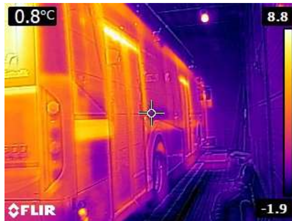
Figure 3 – Gothenburg demonstration: the test in the heat chamber for investigations on heat loss
