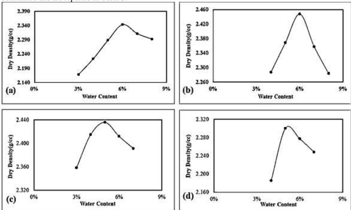
Fig. 3. Dry density Vs water content for (a) gradation I, (b) gradation III, (c) gradation IV and (d) gradation VI
