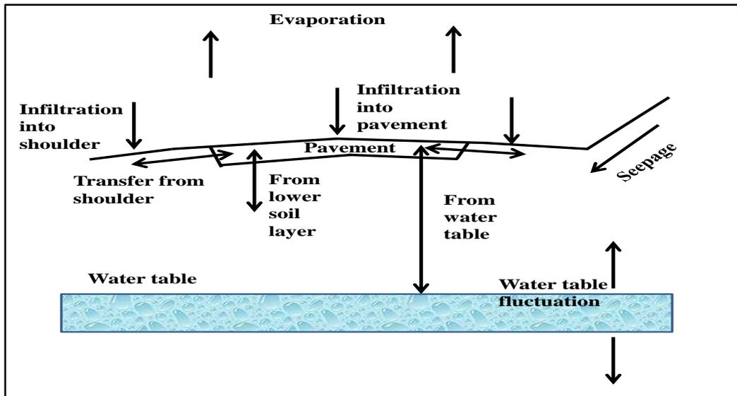
Fig. 1. Moisture movements in the pavement system.
