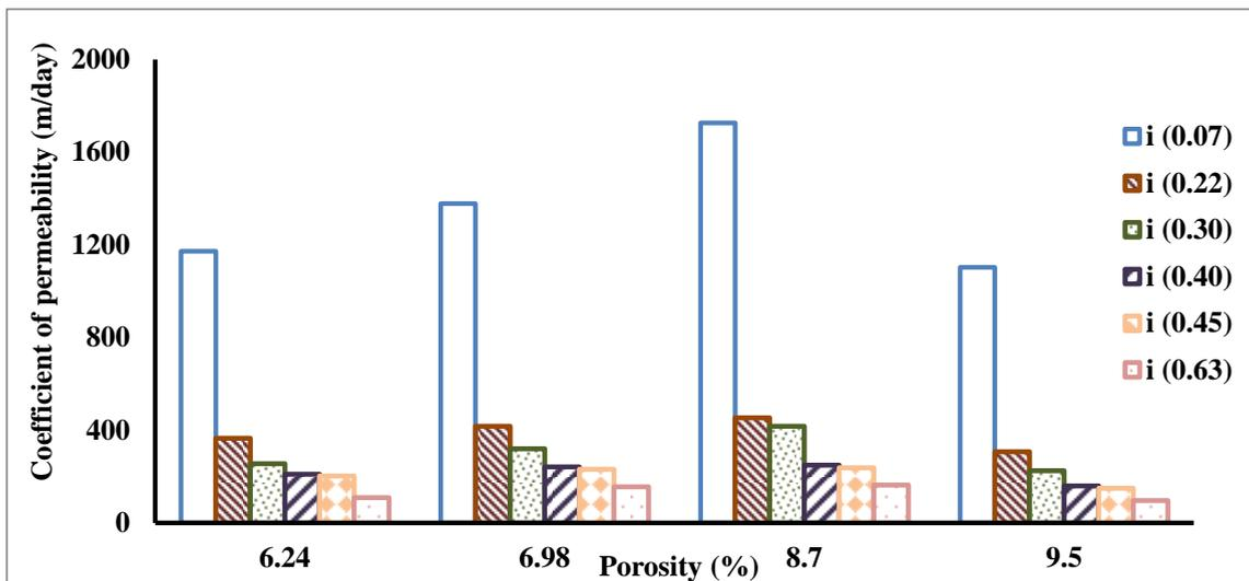
Fig. 7. Porosity versus coefficient of permeability of different gradations at different hydraulic gradient
