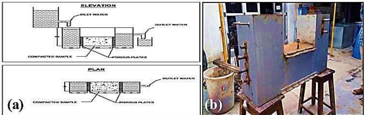
Fig. 4. (a) Sketch and (b) fabricated experimental setup to measure horizontal permeability.
