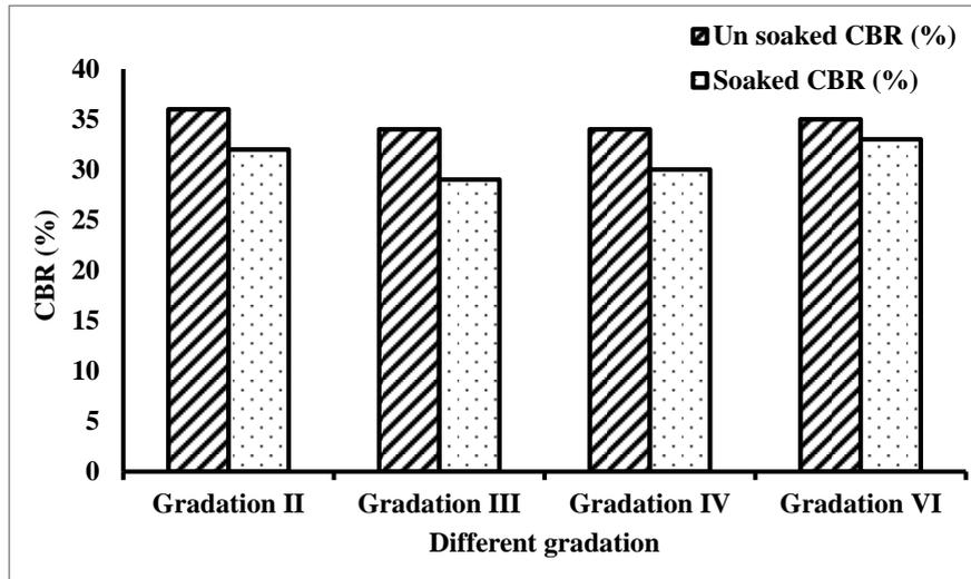
Fig. 5. Soaked and Un-soaked CBR of different gradations
