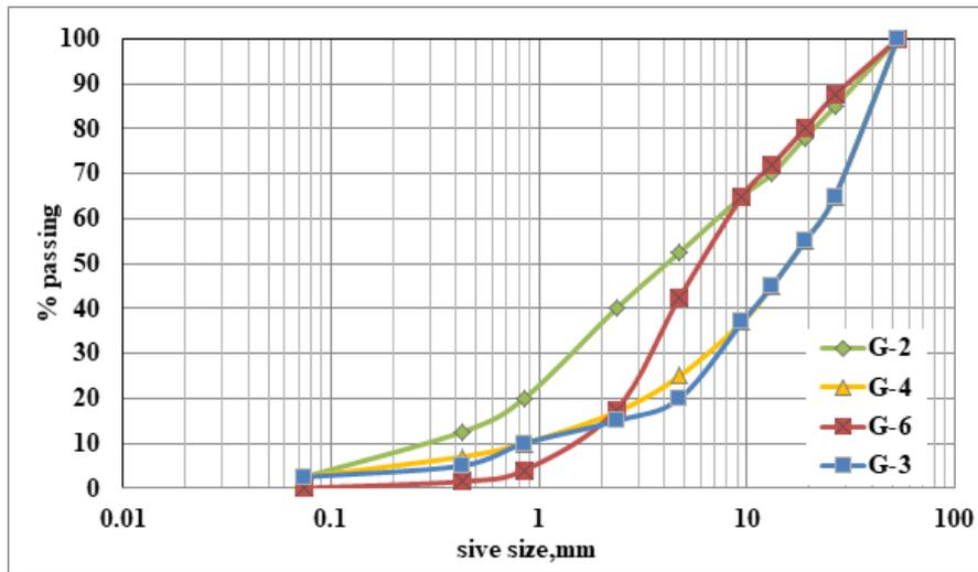
Fig. 2. Gradation of granular subbase materials considered in the present study (MoRTH, 2013)
