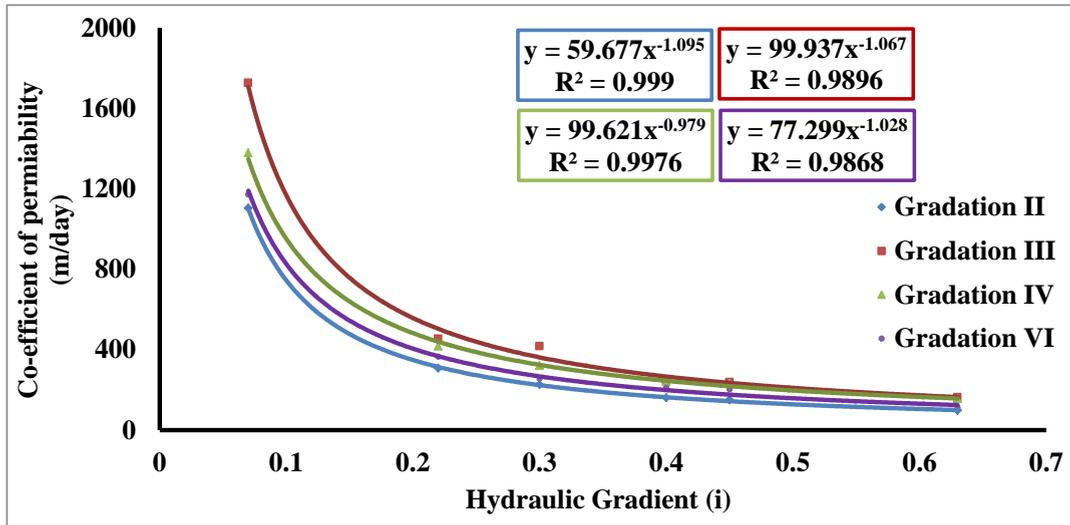
Fig. 6. Coefficient of horizontal permeability at different hydraulic gradient.
