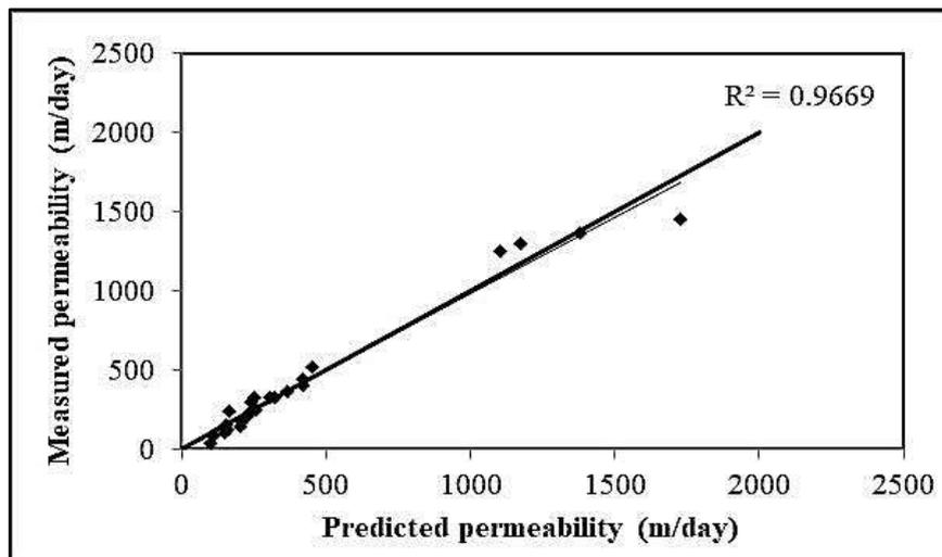
Fig. 8. Predicted permeability versus measured permeability.
