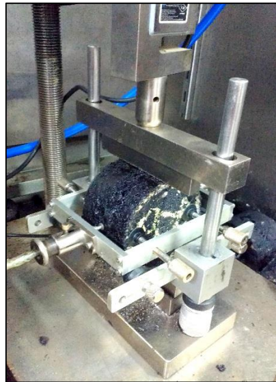
Fig 1: Resilient modulus test setup
