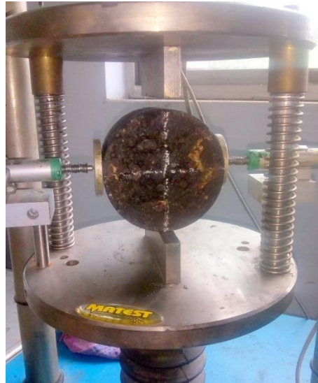
Fig. 4 ITS test set-up
