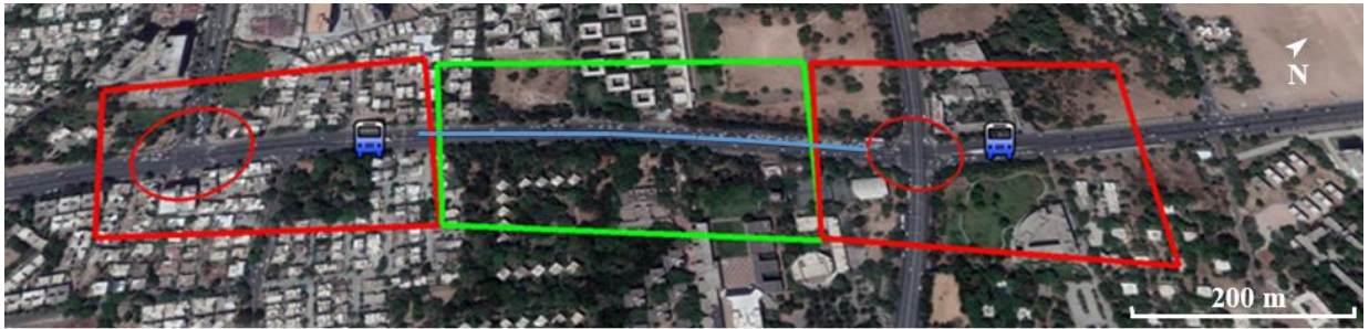
Fig. 6. Variable-length route segmentation for delay variation estimation: Green segment: includes dedicated lane; Red segment: includes intersection and bus stop.
