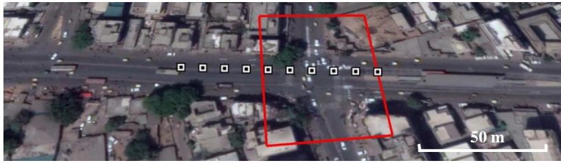
Fig. 5. Grid selection for delay quantification: Red box is the marked intersection and dotted squares represent selected grids based on velocity.
