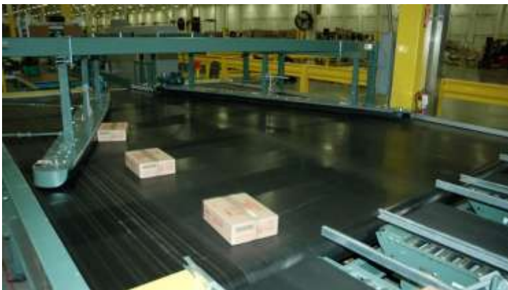
Fig. 13 Typical conveyor aided sorting system
