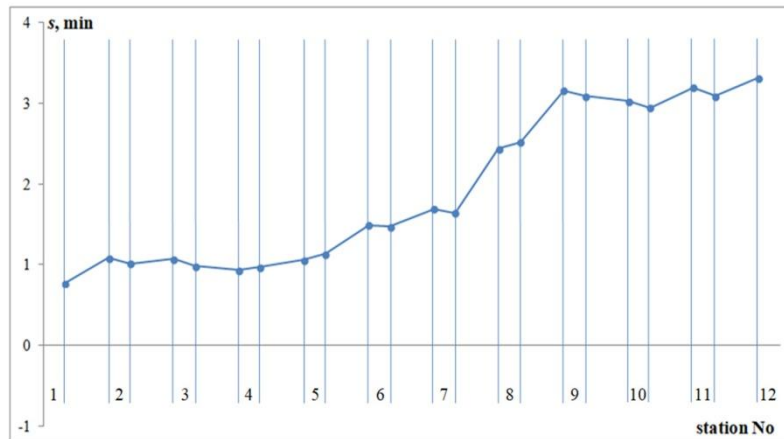
Fig. 6. Behavior of SD of departure and arrival deviations along the route for the suburban line
