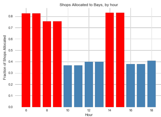
Fig. 6. Fraction of shops allocated to loading bays, by hour. Red denotes peak freight period and blue denotes freight off-peak.
