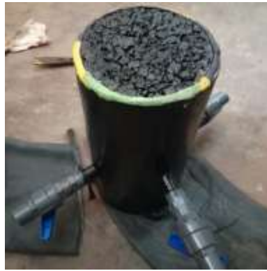
Fig. 4. Sealing the sample with plastic clay
