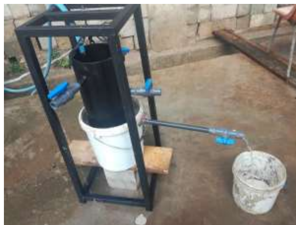
Fig. 2. Permeability apparatus developed for this study
