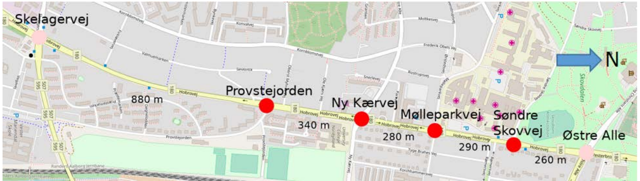
Figure 1 - The six signal controlled intersections in the street Hobrovej and the distance between the intersections. © OpenStreetMap contributors.
