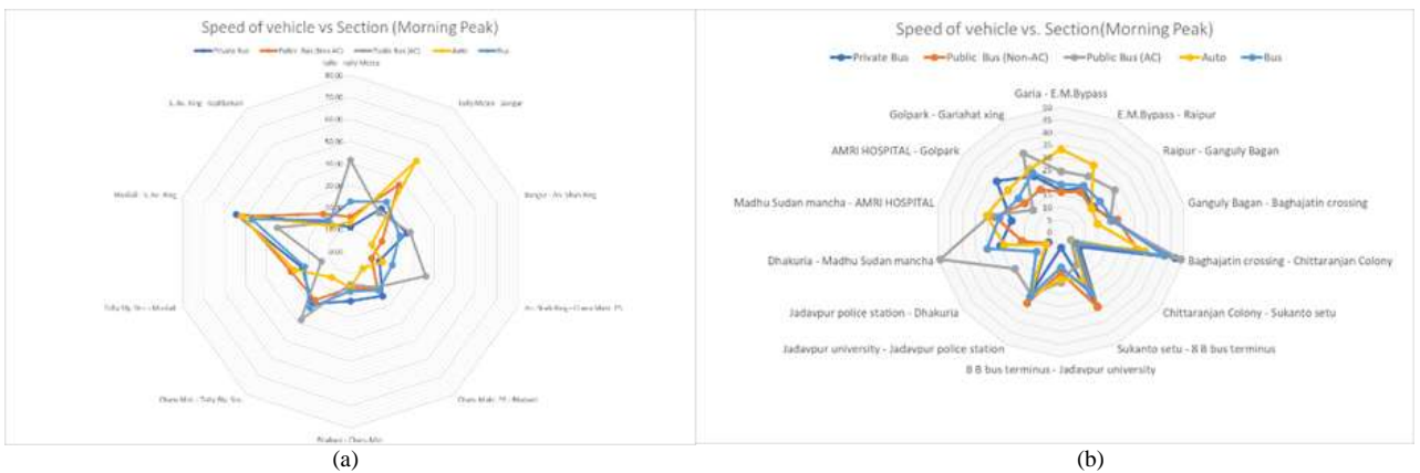
Fig. 6. Average speed (different modes) vs. Stops during peak hours in (a) Corridor A and (b) Corridor B
