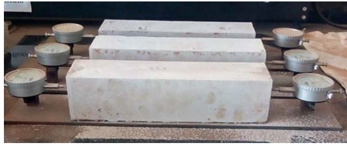
Fig. 6: Drying shrinkage test on the grout
