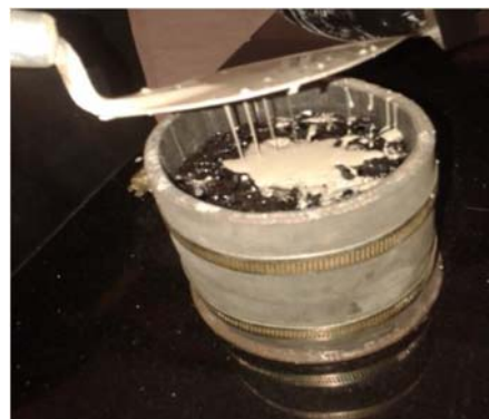
Fig. 2: Process of grouting
