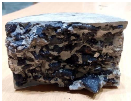
Fig.5: Broken specimen after IDT test
