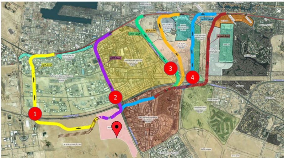
Fig. 1. Alignment options for route 2020 metro extension toward Expo 2020 site [Roads & Transport Authority Dubai].
