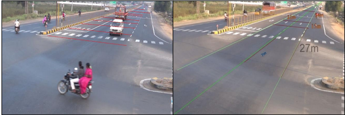
Fig. 4. Speed trap markings to facilitate data extraction
