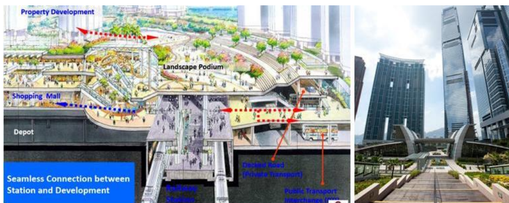
Fig. 5. (a) Conceptual 3-Dimensional section view of Metro station in Hong Kong (b) Kowloon station
