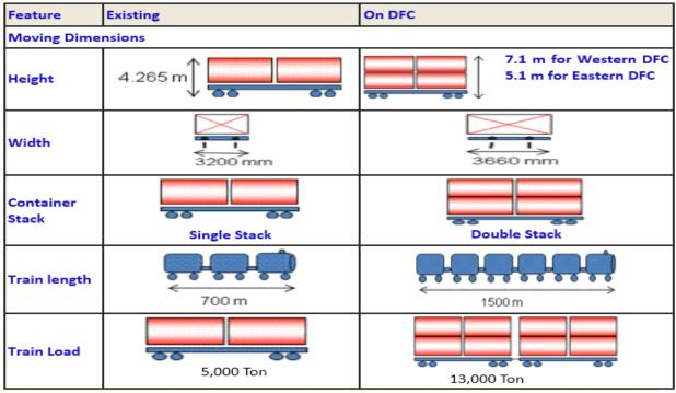
Fig. 3. Upgraded Design Features of DFC [DFCCIL, Salient Features]
