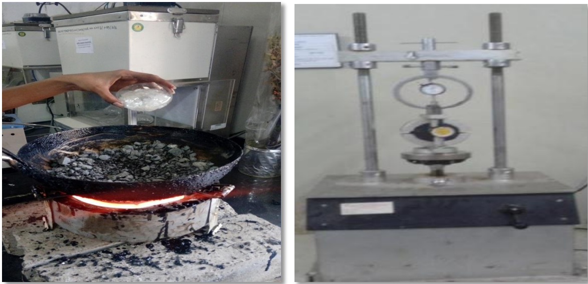
Fig1 Mixing of Shredded Plastic Waste into Aggregates and Arrangements of Samples in Marshall Test set up
