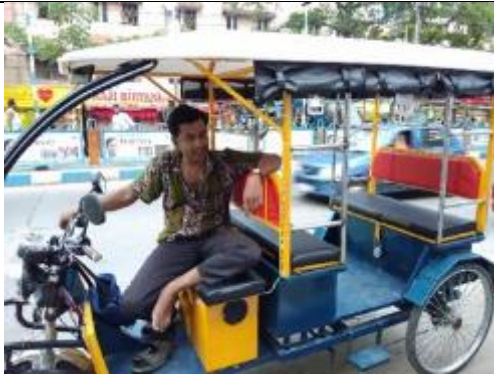
Figure 62. Pedal rickshaw retrofitted with battery – UKM (July 2018)
