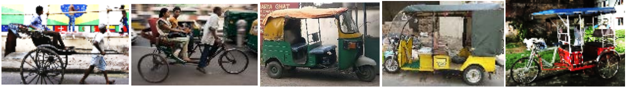
Figure 1. Left to right : Hand-pulled rickshaw, Cycle Rickshaw, Auto-rickshaw (3Wh), Toto, Pedal rickshaw retrofitted with battery or tuntuni
