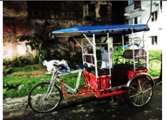
Figure 63. Pedal rickshaw retrofitted with battery – UKM (May 2018)
