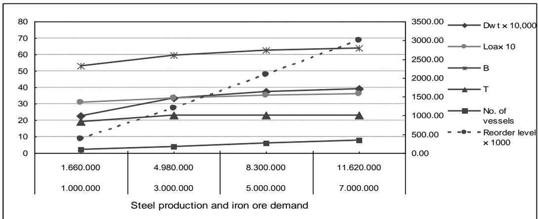
Figure 3- The optimum ship size, main dimensions and the number of vessels for various iron ore demand
