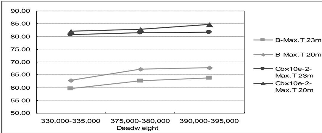
Figure 5-The different breadth and block coefficient of various ship deadweight for draft limitations at 20 meters and 23 meters respectively.
