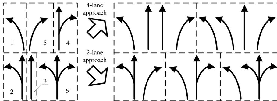
Figure 1 – Illustration of Different Lane-use Patterns
