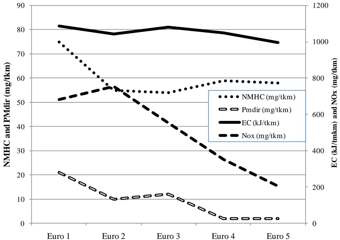
Figure 9: Emissions to air from European HGV engine standards, including prechain emissions
