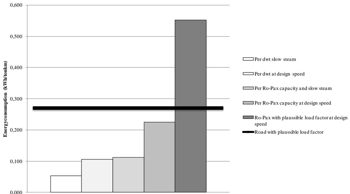
Figure 8: Energy use per tonkm for Ro-Pax vessel vs. Road Transport
