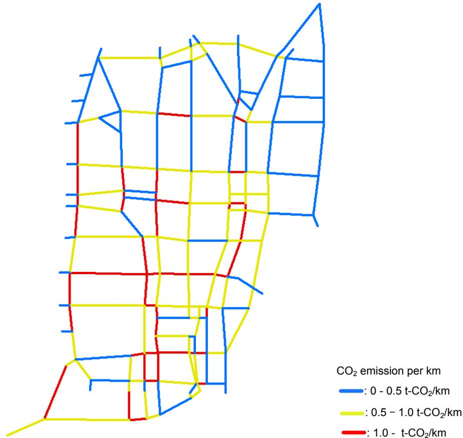
Figure 6 – CO<sub>2</sub> emissions per km for each link
