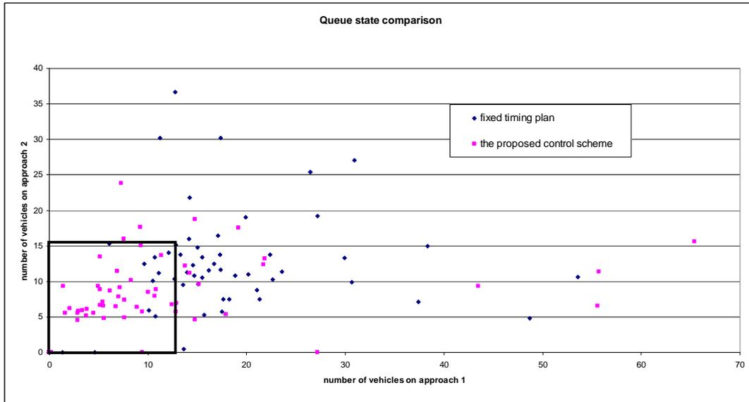
Figure 6 – The resultant queue lengths on the two approaches
