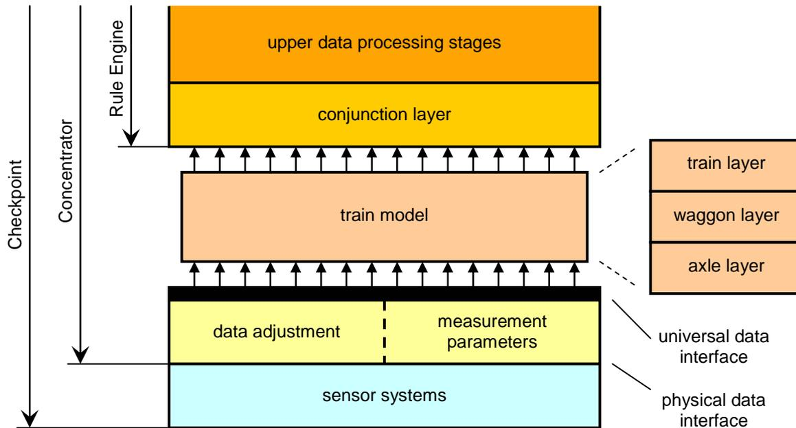
**Figure 3** - Layer model for standardization, data storage and data provisioning
