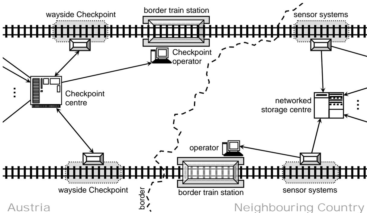
**Figure 6** - System architecture at the border in Scenario 2
