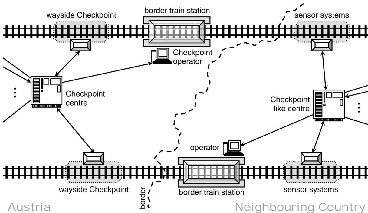
Figure 7 - System architecture at the border in Scenario 3
