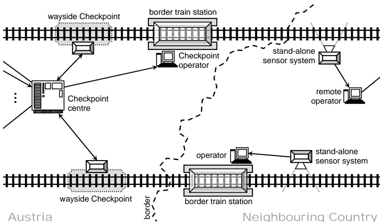
**Figure 5** - System architecture at the border in Scenario 1
