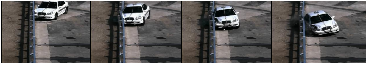
Figure 1 - A vehicle crash test on a roadside barrier
