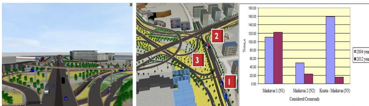
Figure 6 - View on the three-level flyover model fragments in 3D Animation (on the left) and the average delay time in the problem zones for 2004 and 2012 (on the right)
