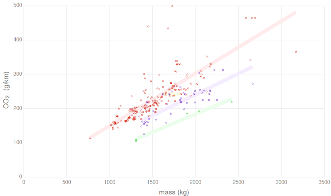
Figure 2: CO 2 emission rates and vehicle mass for new vehicles in Australia, 2008 [green is petrol/electric hybrid, purple is diesel, red is petrol and orange is LPG]
