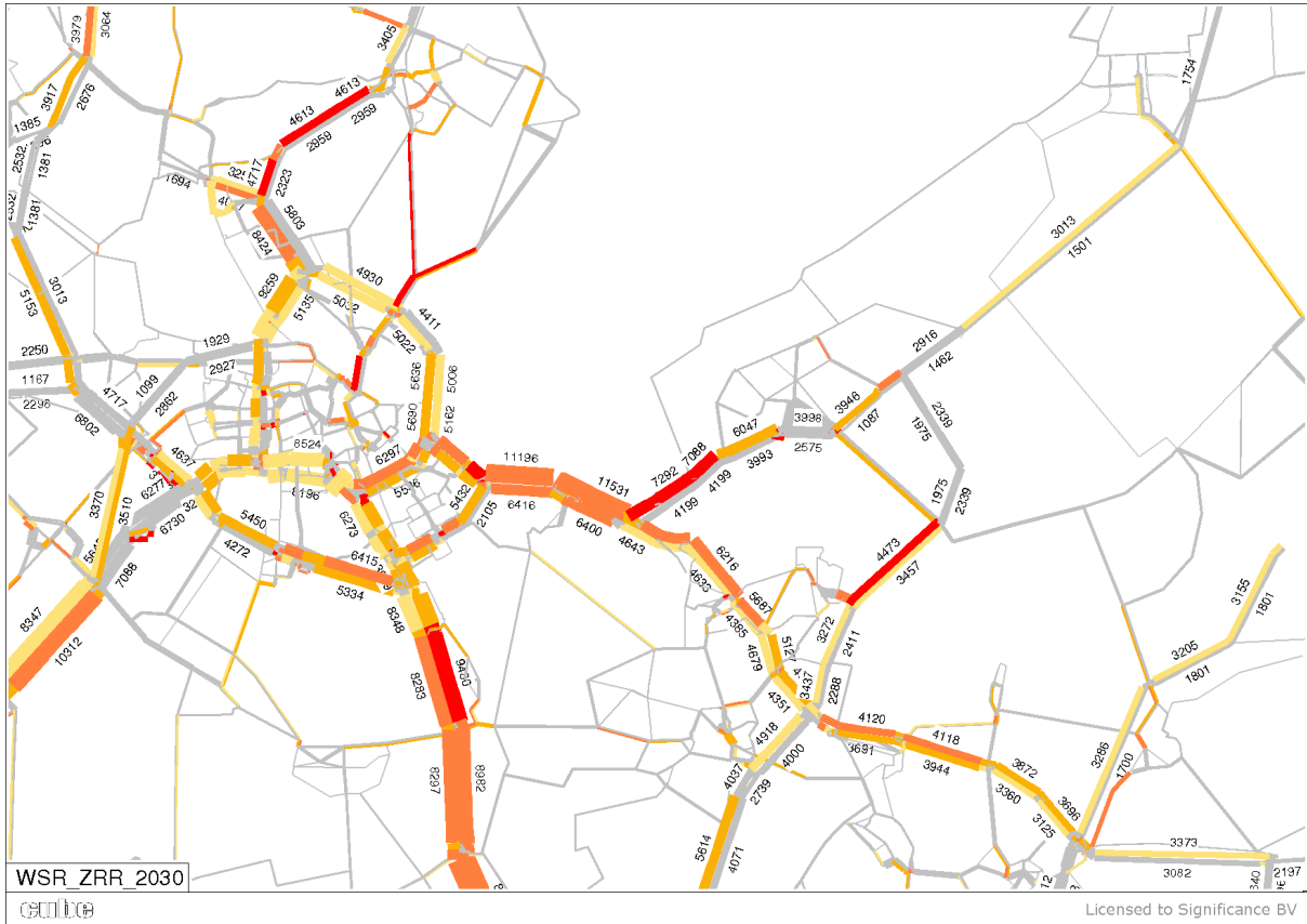
Figure 9: I/C ratio in 2030 in Water Town scenario with IJmeer rail, WITHOUT road pricing scheme
