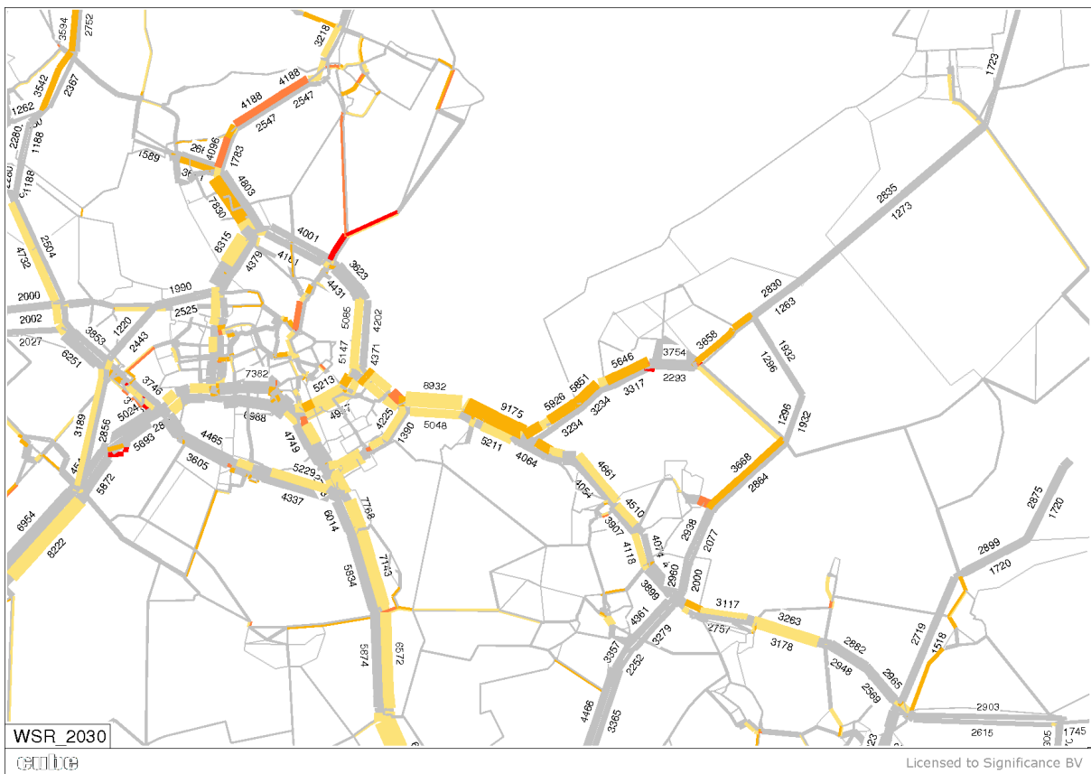
Figure 8: I/C ration in 2030 in Water Town scenario with IJmeer rail WITH road pricing scheme
