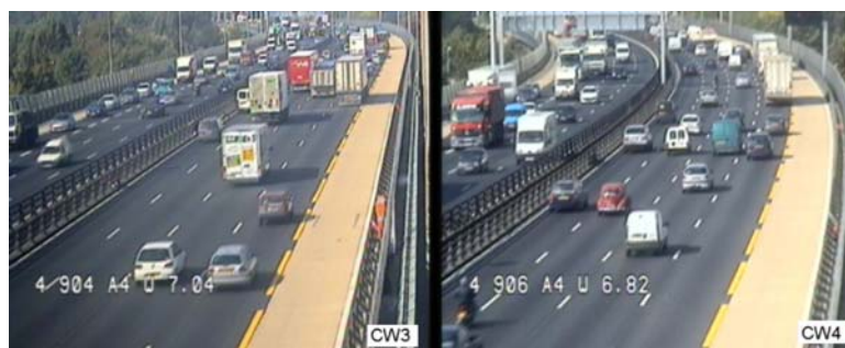
Photo 3. Monitoring of A4-A86 with video AID systems
