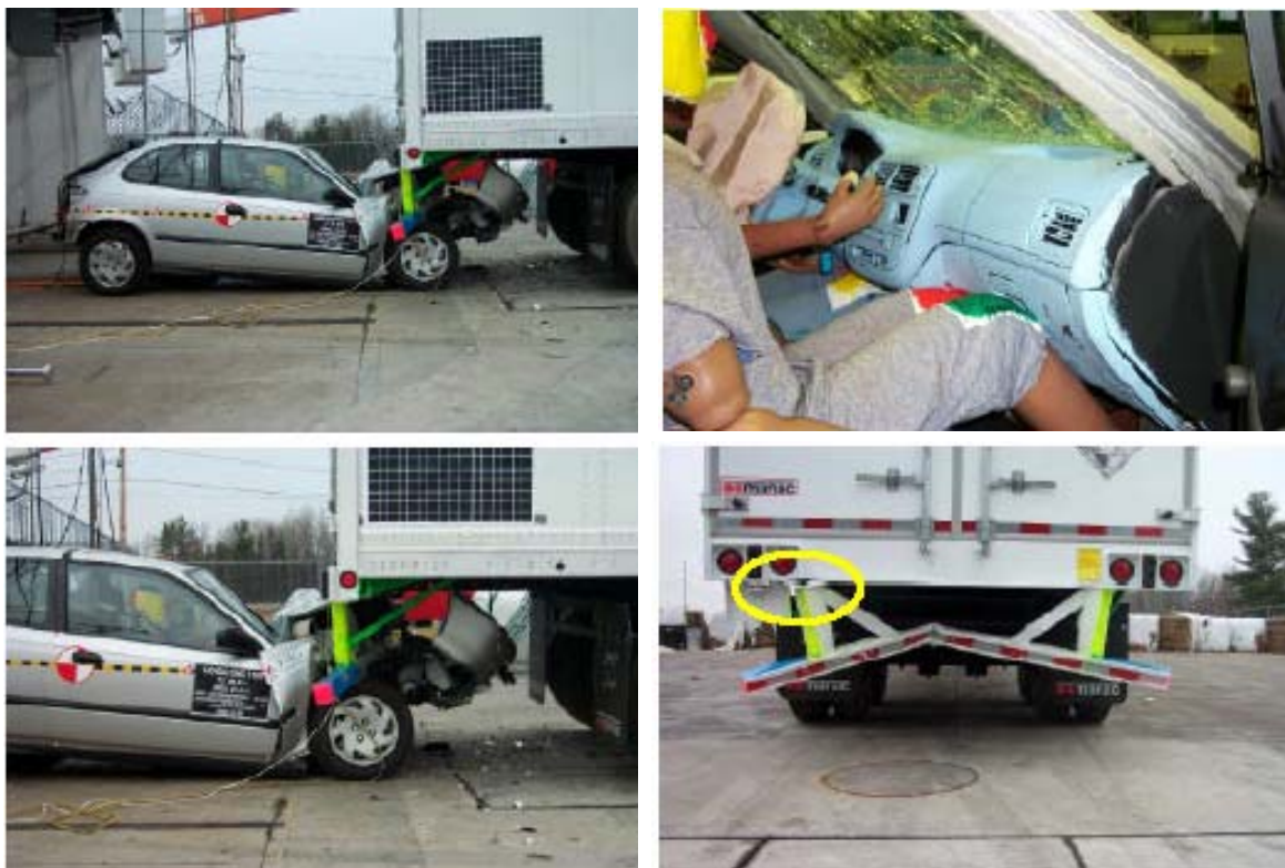
Figure 17. Final crash test on trailer mounted underride guard
