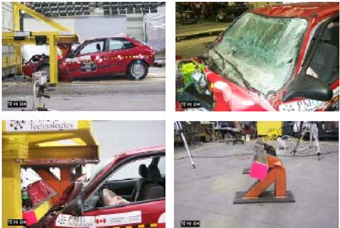
Figure 12. Honda Civic crash test into 480 mm guard at 48 km/h
