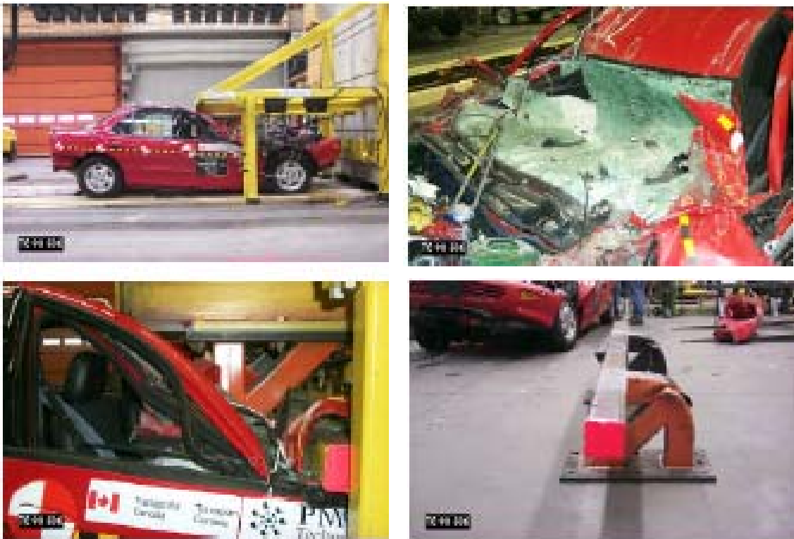
Figure 11. Chevrolet Cavalier crash test into 480 mm guard at 65 km/h
