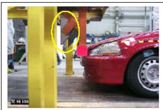
Figure 3. 480 mm displacement limiting guard
