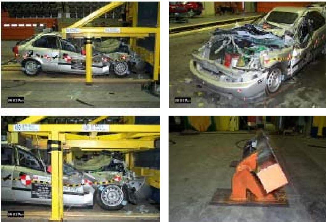
Figure 8. Honda Civic crash test into 560 mm guard at 56 km/h
