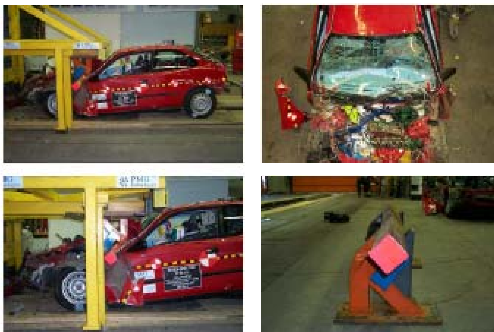
Figure 15. Honda Civic crash test into 480 mm displacement limiting guard at 56 km/h
