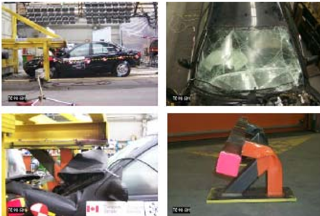
Figure 10. Chevrolet Cavalier cash test into 480 mm guard at 48 km/h
