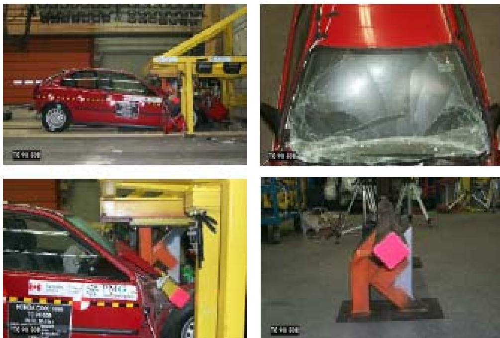
Figure 14. Honda Civic crash test into 480 mm displacement limiting guard at 48 km/h
