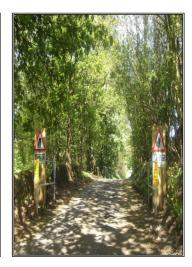
It was agreed by the working group to go ahead with using reclaimed wooden railway sleepers, mounted vertically into the ground in cement. These wooden features would naturally blend with the countryside area, would carry the required information and signing and would be a good use of existing materials.
